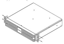
(Figure 2: Mount the Bracket Ears)
