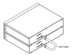
(Figure 9: Parallel the Delta External Battery Packs)
