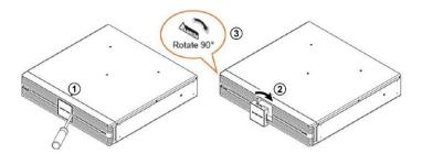
(Figure 5: Rotate the Delta External Battery Pack's
