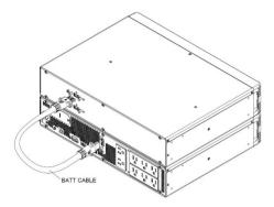
(Figure 8: Connect the UPS and the Delta External Battery Pack)
